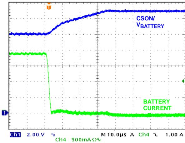
FIGURE 11. BATTERY REMOVAL
