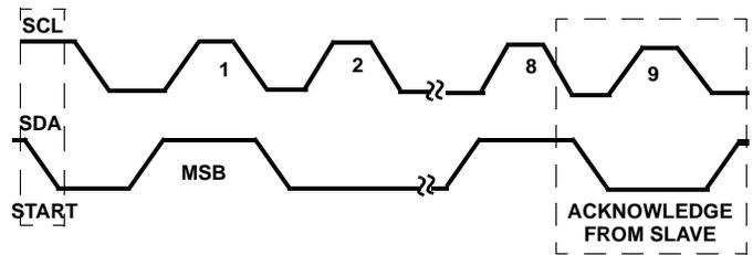
FIGURE 18. ACKNOWLEDGE ON THE I<sup>2</sup>C BUS
