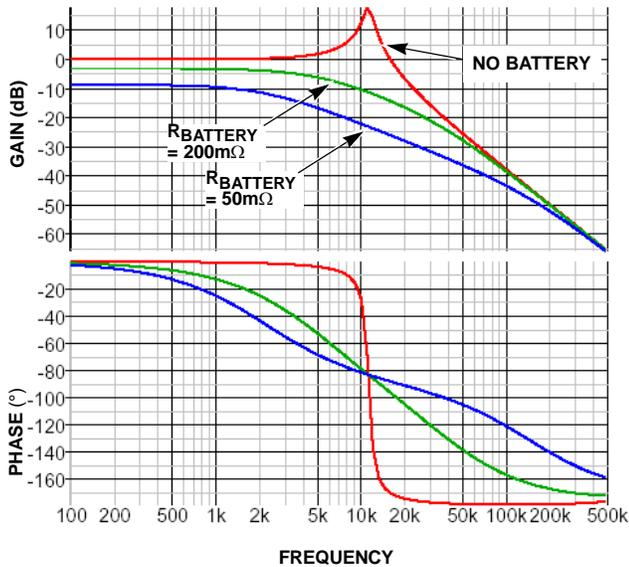
FIGURE 25. FREQUENCY RESPONSE OF THE LC OUTPUT FILTER
