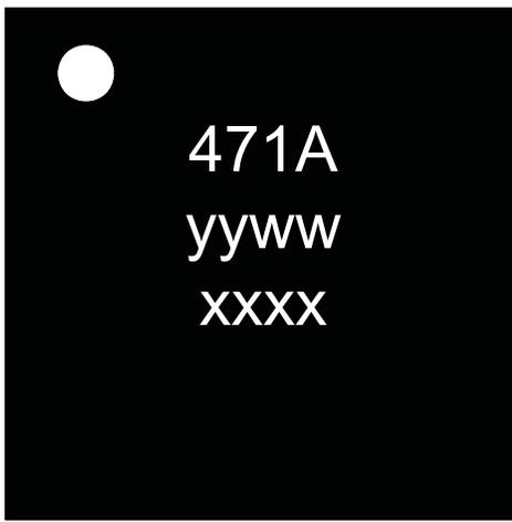
Marking for the 3x3mm MLPQ 16 Lead Package
